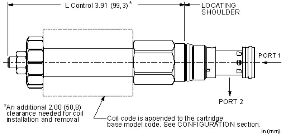
This FLeX Series solenoid-operated, 2-stage, balanced relief cartridge is a pressure regulating valve.
